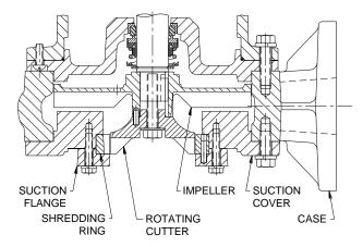
**Grinder Pumps** – To 100 GPM. Solids are reduced to a 3/8-inch diameter by the grinder cutter and shredding ring components. The 3/8-inch solids are then pumped by the impeller into the discharge line. The impeller is sized to efficiently pump the slurry at flows and pressures determined by the system design.
